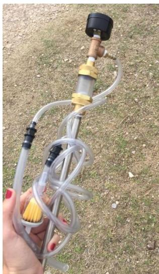
**Figura 29. Sonda Soil Gas Probe (User Manual, 2016)**
