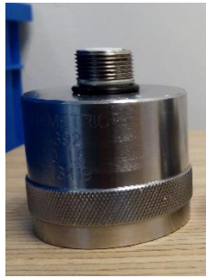
Figura 69. Transductor V392 NDT de 1 MHz
