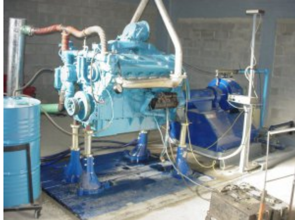
Figure 5: An example of an engine test stand used to analyze Diesel engine's parameters
