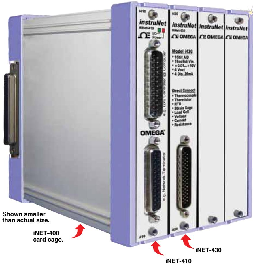
iNET-400 measurement modules have universal inputs that enable one to directly connect each channel to one of: thermocouple, thermistor, strain gage, load cell, counter/timer, RTD, voltage, current, resistance and accelerometer.
