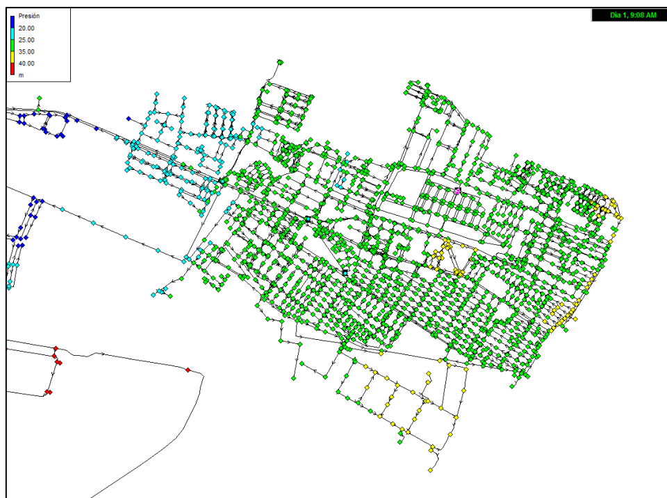
Figure 4-7. Pressure map of the network of Port Sagunt after the improvements
