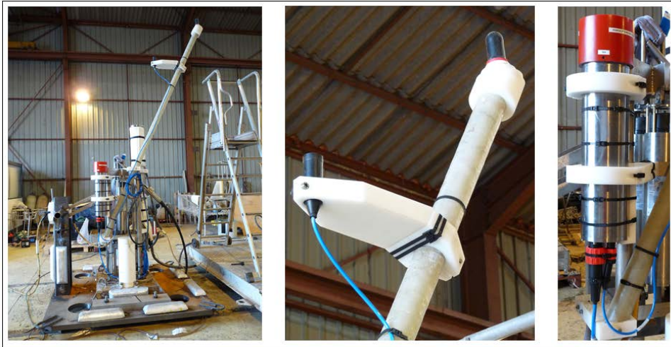
Figure 7. Picture of the anchor of the Instrumentation Line of ANTARES showing the final integration of the transceiver. Details of the FFR-SX30 hydrophone with its support and of the titanium container housing the SEB are also shown.
