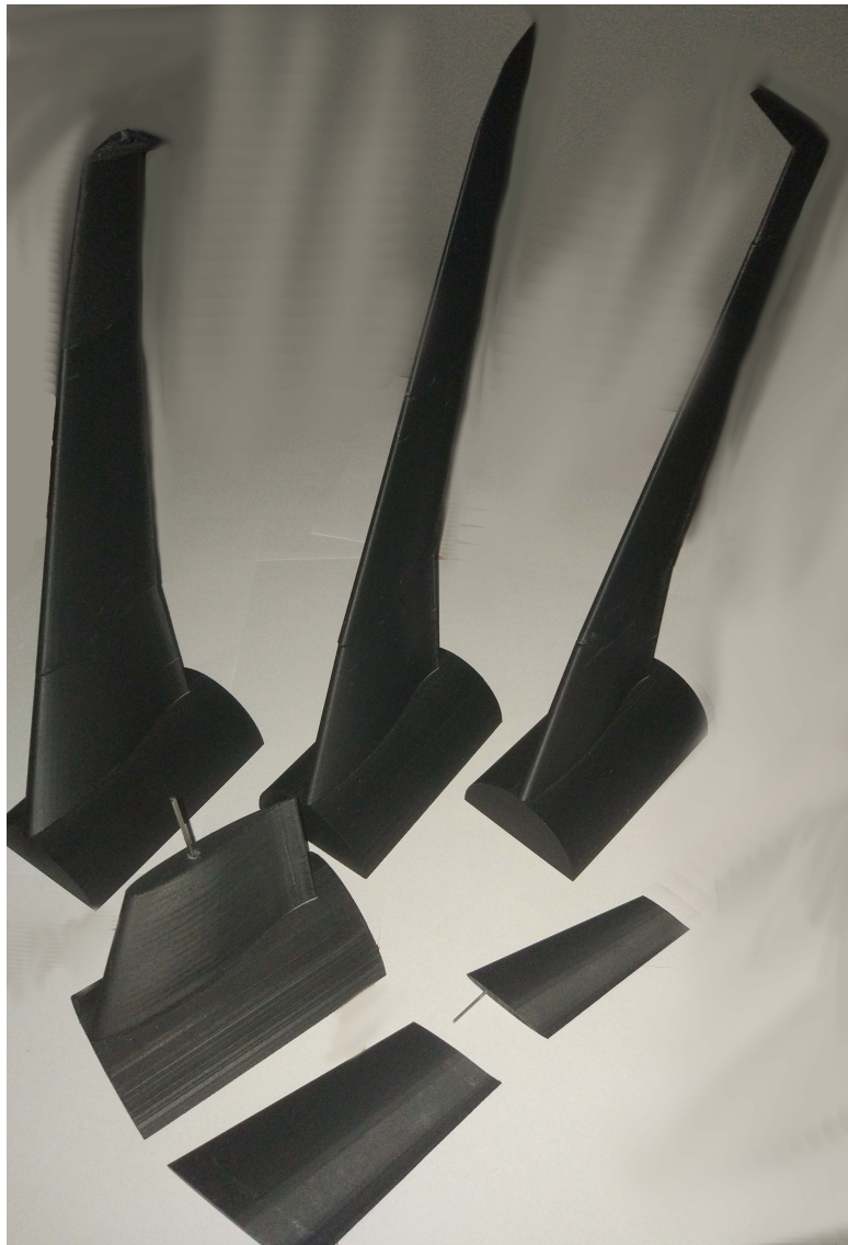
Figure 4.3: No winglet, blended and endplate models built. Raked model showing the inner supporting structure.
