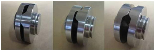
Figure 2. The AM2 masticatory chamber. It is a cylindrical cavity whose two ends are formed by the stationary “maxillary disk” and the moving “mandibular disk”; this can move back and forth along and rotate around the central axis of the cylinder. Both AM2 disks are shown in the different positions during operation.
