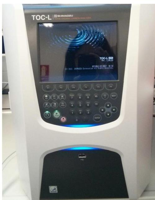
*Figura 11. Total organic carbon analyzer TOC-L de Shimadzu*
