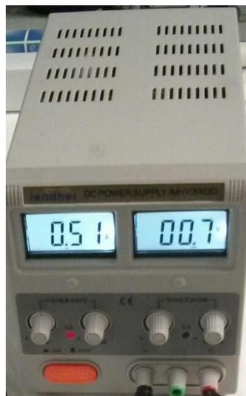
Figura 4. Fuente DC power supply IMHY 3003D de Lendher x2
