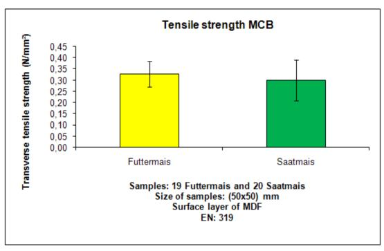
**Figure 32:** Tensile strength (N/mm<sup>2</sup>) from samples of core layer made with Futtermais and surface layer of MDF, and samples made with core layer of Saatmais and surface layer made of MDF. Size of samples is (50x50x40) mm. Number of samples: 19 samples with core layer of Futtermais and surface layer of 6 mm MDF, and 20 samples with core layer of Saatmais a surface layer of 6 mm MDF. Following the standard ÖNORM EN 319
