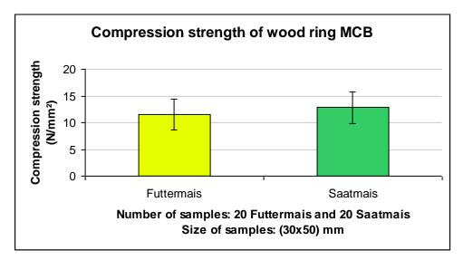
Figure 36: Perpendicular compression strength of wood ring, comparing samples of growing-maize (Saatmais) cobs and food-maize cobs (Futtermais). Units: N/mm<sup>2</sup>.
