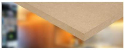
Figure 14: Sample of light MDF board (<u>www.Spanogroup.be</u>)
