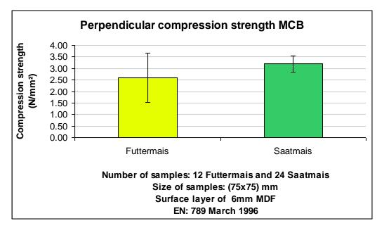
Figure 33: Perpendicular compression strength (N/mm<sup>2</sup>) from samples of core layer made with Futtermais and surface layer of 6mm MDF, and samples made with core layer of Saatmais and surface layer made of MDF. Size of samples is (75x75x40) mm. Number of samples: 12 samples with core layer of Futtermais and surface layer of MDF, and 24 samples with core layer of Saatmais a surface layer of MDF. Following the standard ÖNORM EN 789 March 1996
