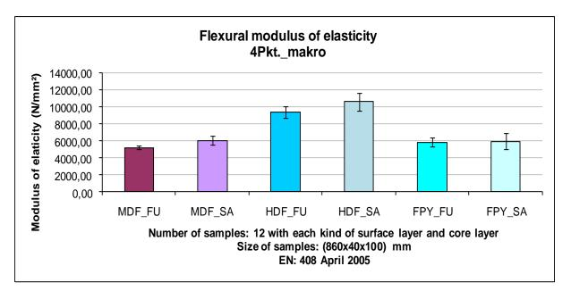
Figure 37: Flexural modulus of elasticity 4Pkt.\_makro (N/mm<sup>2</sup>). Number of samples:
