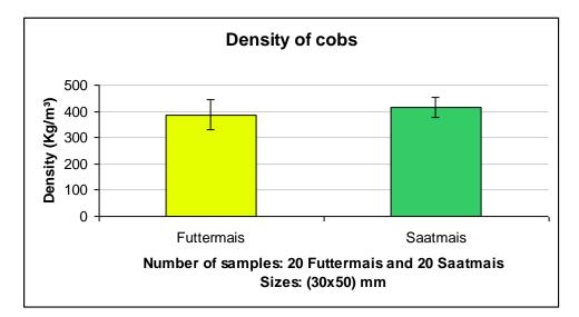
**Figure 31:** Density of cobs (Kg/m<sup>3</sup>) from samples of Futtermais and Saatmais. Size of each sample: (30x50) mm. Number of samples: 20 of Futtermais and 20 of Saatmais
