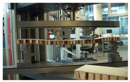
Figure 28: Determination of the bending strength by four points bending until the sampled is collapsed.
