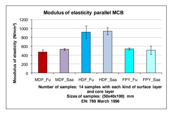
**Figure 41:** Modulus of elasticity parallel of MCB samples (N/mm<sup>2</sup>). Number of samples: 14 with each kind of surface layer and core layer. Samples of a surface layer of MDF
