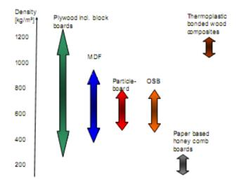
Figure 3: Density ranges of different panel types (Michanickl, s.a.)
