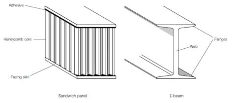
Figure 9: Shows the construction of a sandwich panel compared to I-beam (Hexcel Composites 2000)
