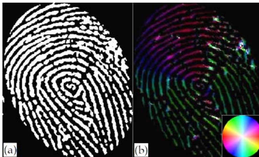
Figure 2.30. Tensor scale 2D method applied to a binarized fingerprint (a). Representation of the main orientations using HSV color coding applied to the 2D tensor scale results (b).
