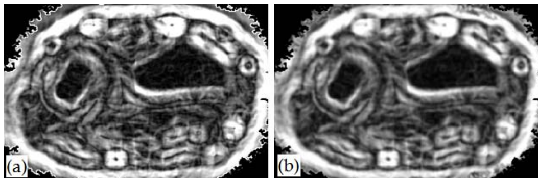
Figure 2.6. In (a), results after the application of a 3x3 rank filter. Contours are depicted with a high sensitivity. In (b), a better contours uniformity is obtained after the application of an average filter with a 3x3x3 mask.
