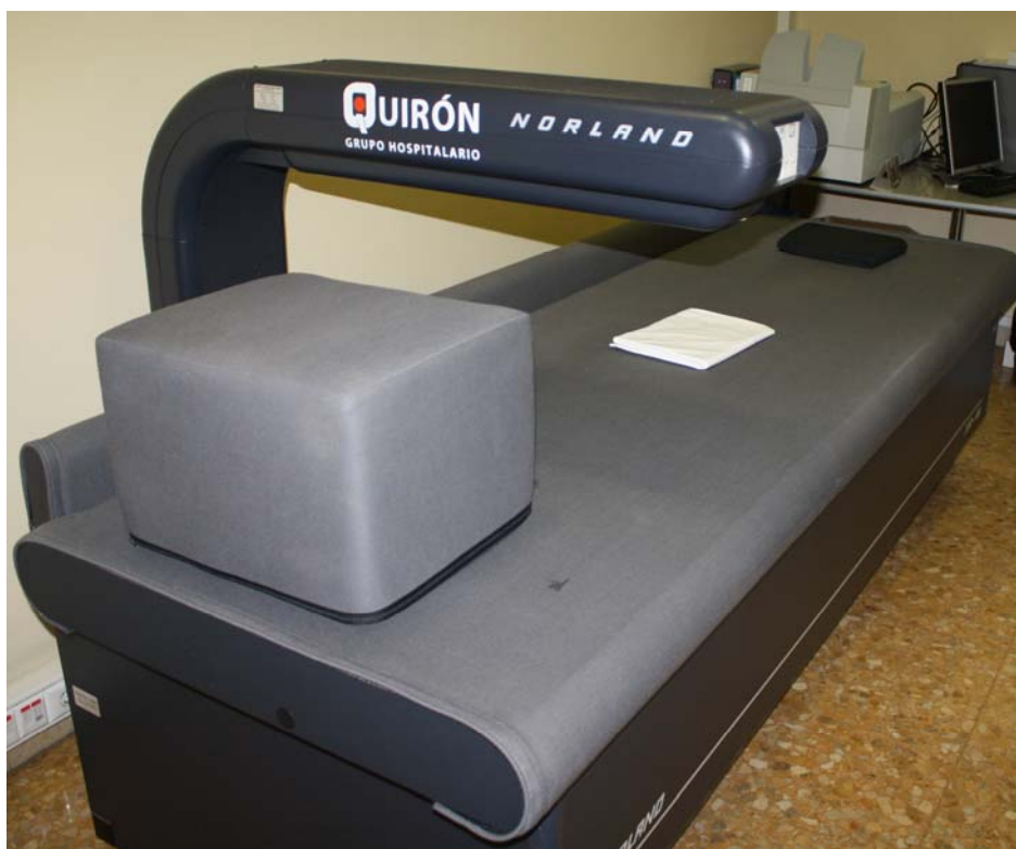
Figure 1.5. Dual-Emission X-Ray Absorptiometry (DXA) scanner (Norland, Fort Atkinson, WI) for Bone Mineral Density (BMD) quantification at Quirón Valencia Hospital.
