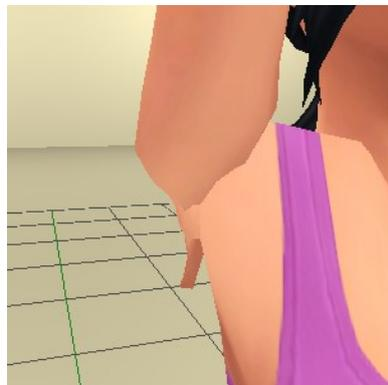
**IMAGEN 27: PINZAMIENTO DE LA MALLA AL DEFORMARSE SEGÚN EL ESQUELETO.**
