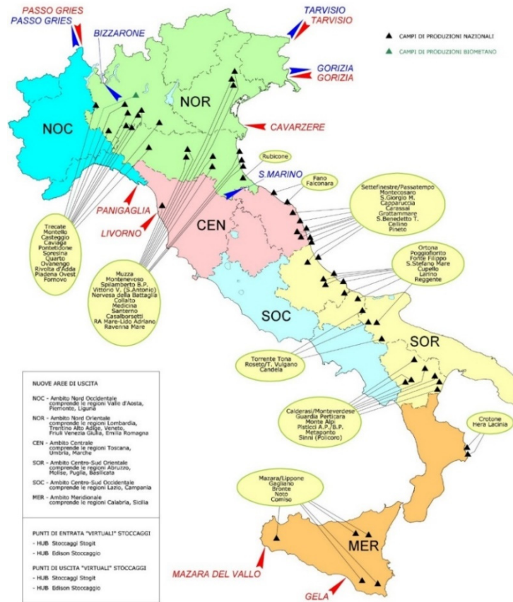
Figure 3.37. Natural gas production sites in Italy and national entry and exit points (Source: SNAM rete gas)
