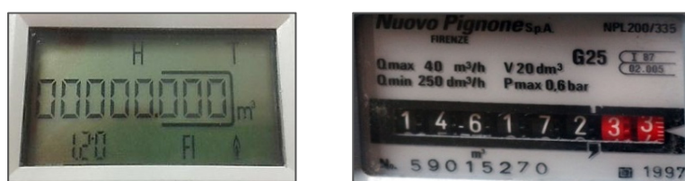
Figure 4.9. Electronic display vs a traditional totalizer
