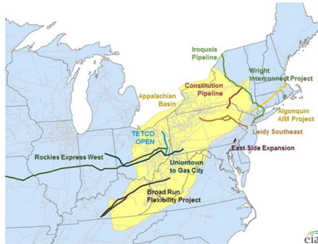
Figure 3.40. Implementation of new pipelines in USA (Source: New pipeline projects increase Northeast natural gas takeaway capacity, January 28, 2016)
