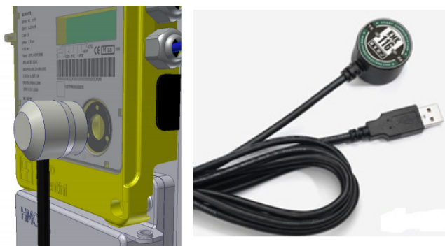
Figure 4.10. Optical port connected through a ZVEI probe (Source: www.florentini.com – www.marcom.com )
