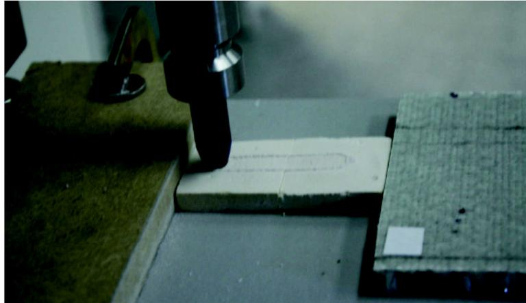
Imagen 8.3. TABER<sup>®</sup> Linear Abraser Modelo 5750 NEURTEK Instruments.
