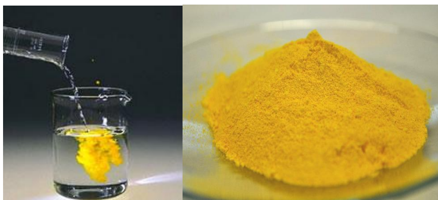
Figure 6.1.1.3.6 Cadmium sulphide precipitation reaction (left) and cadmium yellow used in this research project (right).
