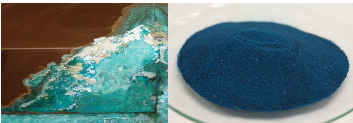
Figure 6.1.1.3.3 Copper plates exposed to acetic acid (left) and verdigris used in this research project (right).
