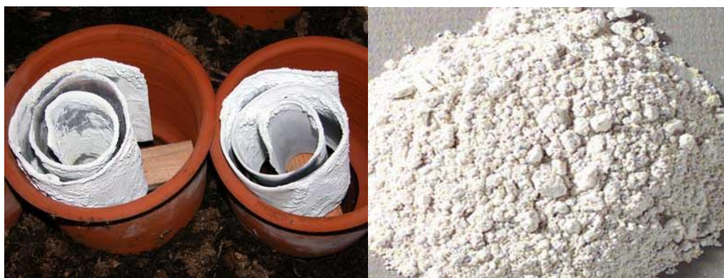
Figure 6.1.1.3.4 'Stack' process, corrosion on the lead coils (left) and lead white used in this research project (right).
