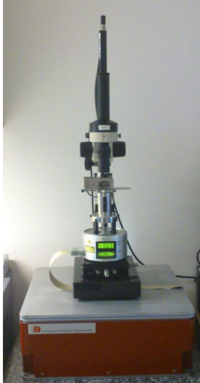
Figure 7.2.4.2. AFM-nanoindentation equipment used in this study.
