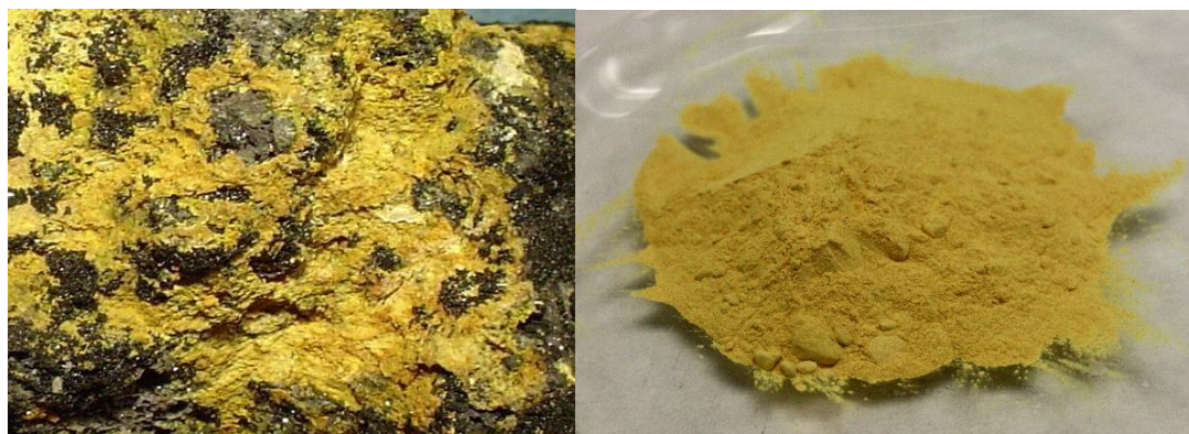
Figure 6.1.1.3.2 Mineral massicot (left) and massicot pigment used in this research project (right).
