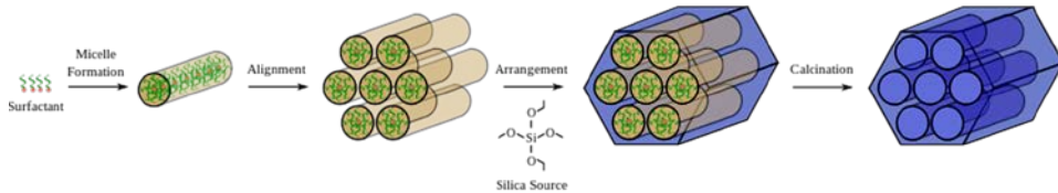
Figure 3-3. Synthesis of mesoporous silica-based materials from surfactant micelles to an ordered hexagonal porous structure (MCM-41 type material).
