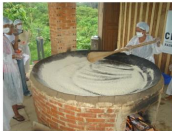
Figure 7: Roasting of fish flour.
