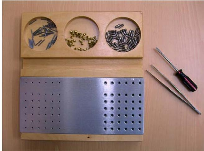
Figura 21. Crawford Small Parts Dexterity Test
