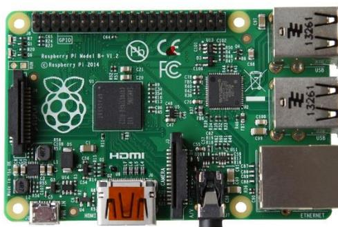
Figura 4. Raspberry Pi. [https://en.wikipedia.org/wiki/Raspberry\\_Pi](https://en.wikipedia.org/wiki/Raspberry_Pi)
