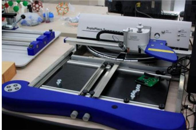
**Figura 67 - Máquina Pick and Place de LPKF [19]**
