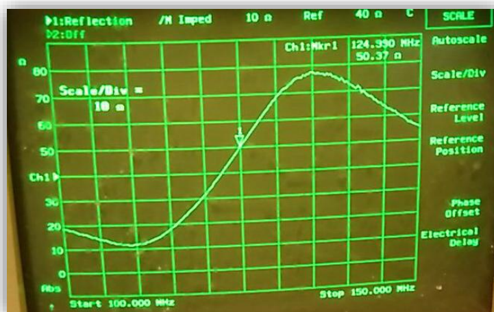
Fig 38. LNA output impedance: magnitude
