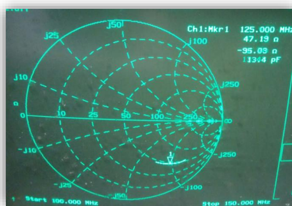
Fig 29. Signal generator output impedance
