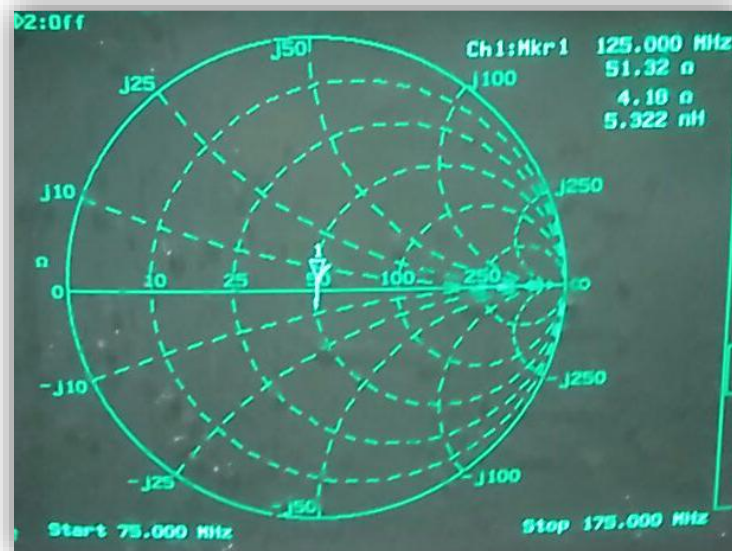
Fig 31. AC load input impedance
