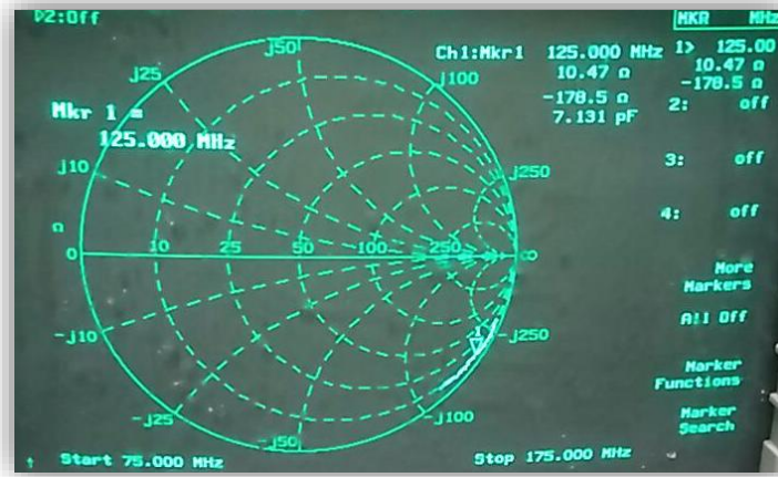
Fig 37. Output impedance of the current buffer
