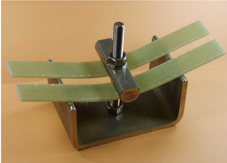
Figure 1. Device to apply the service stress to samples submerged in sea water medium.
