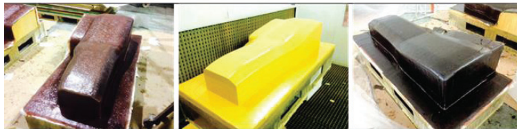
Fig. 8. Manufacturing process of monocoque mold from CAD part to final mold. Photos by a project's partner, Sinergia Racing Group.
