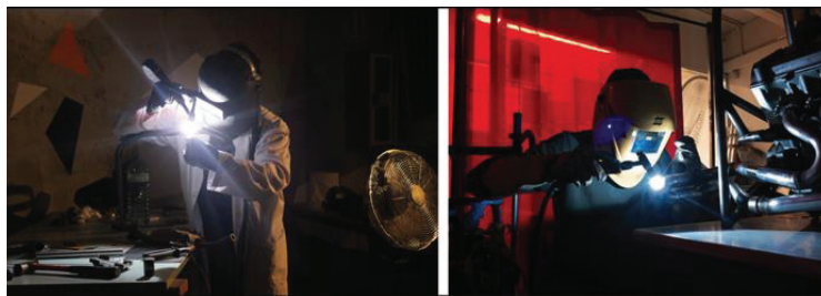
Fig. 11. Welding some steel parts of the race car
