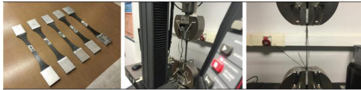
Fig. 7 Process of characterization of Gurit's carbon fiber material
