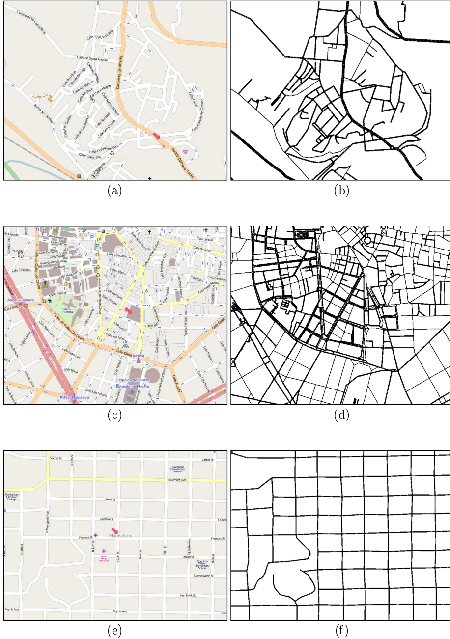
Figure 7.16: Scenarios used in our simulations: (a) fragment of the city of Teruel (Spain) obtained from OpenStreetMap, and (b) the same fragment as a street graph in SUMO. (c) Fragment of the city of Valencia (Spain) obtained from OpenStreetMap, and (d) the same fragment as a street graph in SUMO. (e) Fragment of the city of Manhattan (KS) obtained from OpenStreetMap, and (f) the same fragment as a street graph in SUMO.
