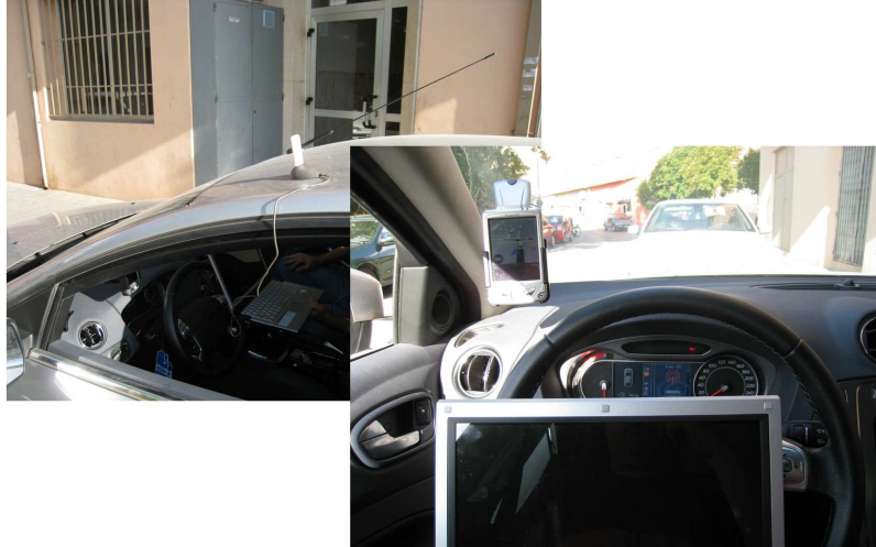
Figure 7.3: Images of the experiment to determine the radio signal attenuation due to distance between vehicles.
