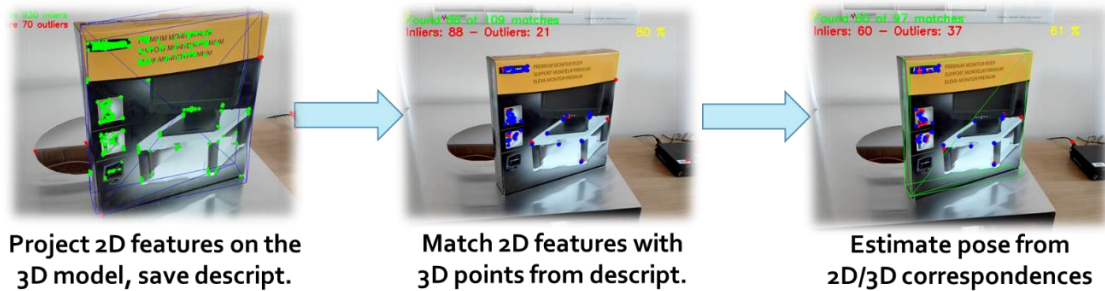
Figure 26 - Tracking workflow with images
