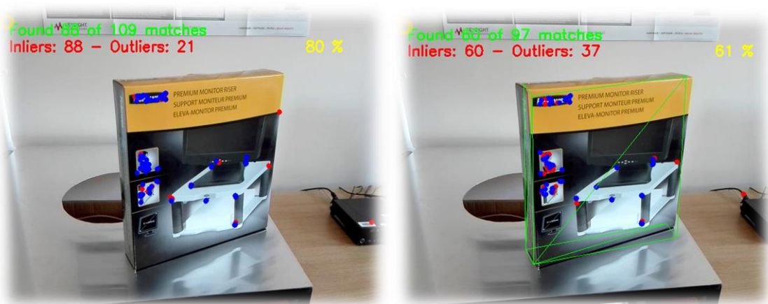
Figure 31 - Feature matching (left) and Pose estimation (right) examples
