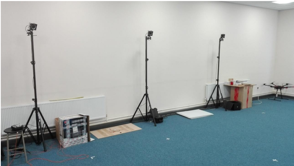
Figure 21 - View of the laboratory's OptiTrack environment
