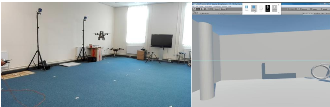
Figure 32 - Drone tracking module, flight test (left), Unity view (right)
