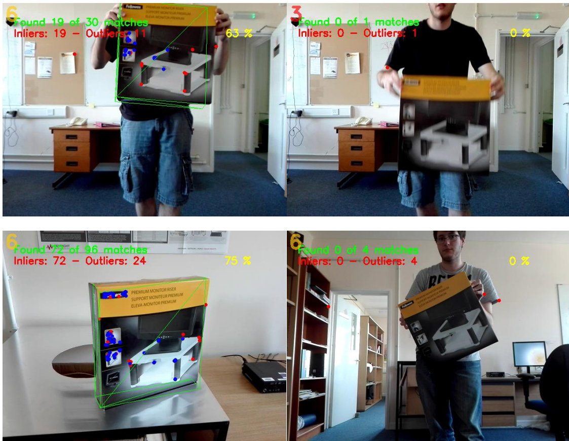
Figure 34 - Tracking examples with "monitorbox", success (left) & failure (right)
