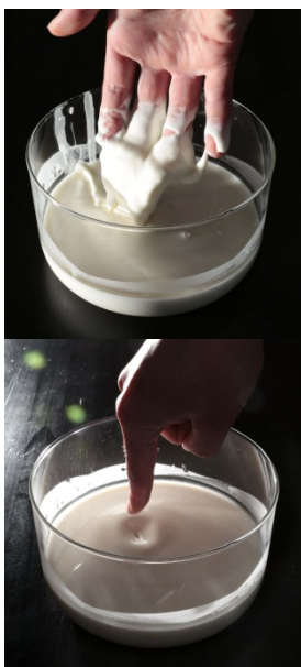
Figure 5. Investigation of the flow behaviour of non-Newtonian fluids
