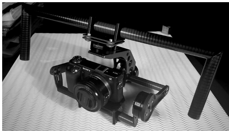
Figure 7. Gimbal 1 for bigger cameras in helicopters
