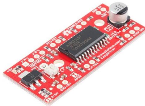
Figura 20. Drive motor EasyDriver [33].
