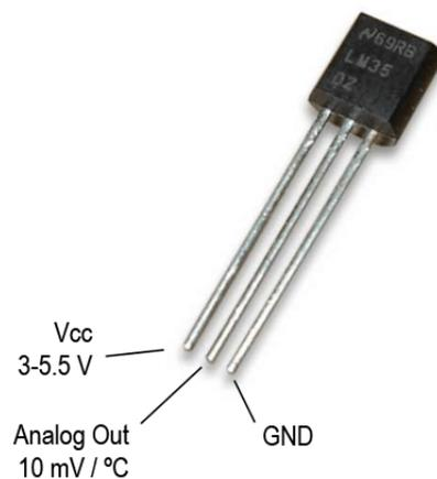
**Figura 14:** Sensor Temperatura LM35
