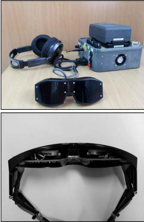
Fig. 2. System components. The laser was assembled on a pair of glasses.
