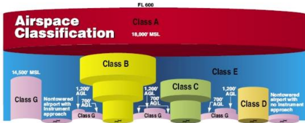
Figure 7: Types of controlled airspace (adapted from the FAA webpage, accessed the 02/06/2017. www.faa.gov )
