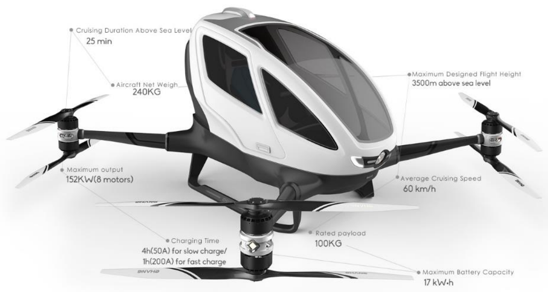
Figure 4. EHANG 184 design and specifications (Adapted from Ehang, Inc. Official website, http://www.ehang.com/ehang184/ , accessed on 05/07/2017).
