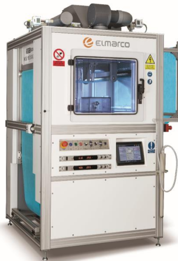
Figure 7. Industrial-scale electrospinning equipment. a) Nanospinner 416, produced by Inovenso Ltd. Reproduced with permission from Inovenso Ltd. b) Nanospider™, produced by Elmarco. Reproduced with permission from Elmarco.
