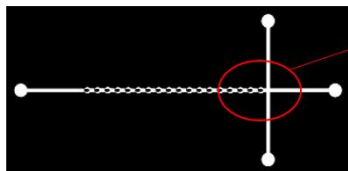
Figure 1. Schemes and corresponding micrographs of the three different designs of microfluidic mixing devices used in this work. The microchannels are 200 μm wide and 50 μm deep.
