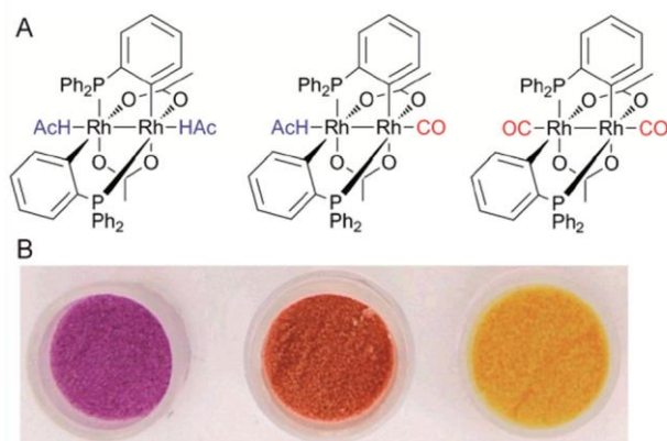
Figure 3.4. Colorimetric detection of CO via binuclear rhodium complexes. (A) Basic structure of the complexes (HAc = \text{CH}_3\text{CO}_2\text{H} ). (B) The photograph shows ([\text{Rh}_2\{(m\text{-CH}_3\text{C}_6\text{H}_3)\text{P}(m\text{-CH}_3\text{C}_6\text{H}_4)_2\}_2(\text{O}_2\text{CCH}_3)_2](\text{CH}_3\text{CO}_2\text{H})_2) adsorbed on silica gel in the absence (left) and presence of 8 ppm (middle) and 2000 ppm (right) of CO in air. Adapted with permission from ) M.E. Moragues, J. Esteban, J.V. Ros-Lis, R. Martínez-Máñez, M.D. Marcos, J. Soto, F.Sancenón, J. Am. Chem. Soc. 2011 , 133, 15762. Copyright © 2011 American Chemical Society.
