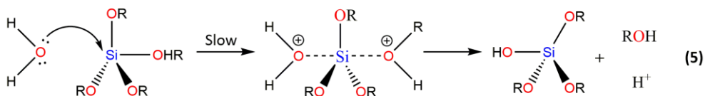
Scheme 1.2. Hydrolysis mechanism of an alkoxy silane using acidic catalyst.
