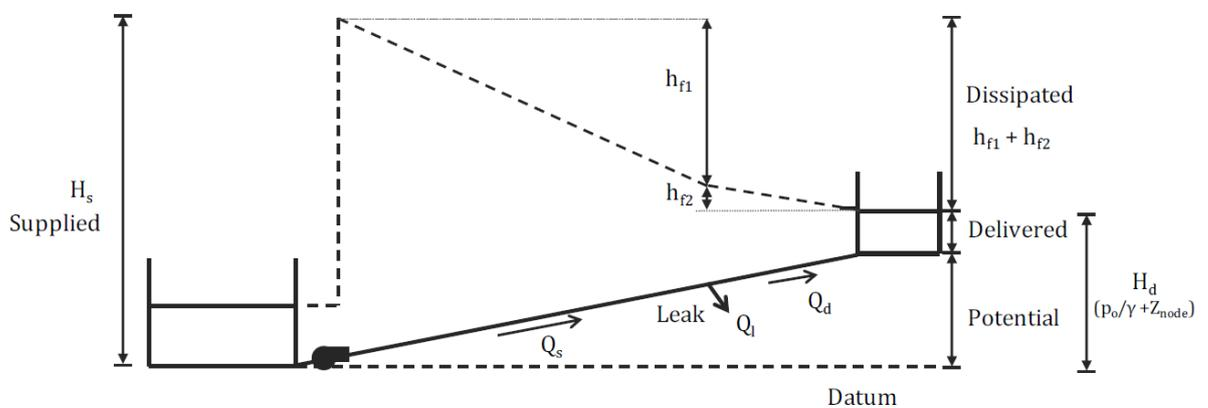
**Fig. 1.** Schematic representation of a simple system, including the main energy concepts.
