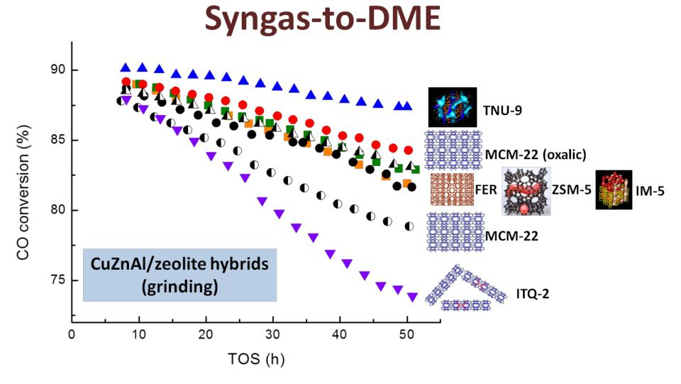
Deactivation inhibited for zeolites with low external surface areas and Al-depleted surfaces
