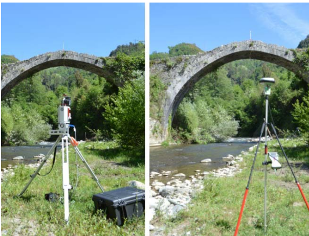
Figure 12: Survey of the Hannibal Bridge with Laser Scanner and GNSS receiver.
