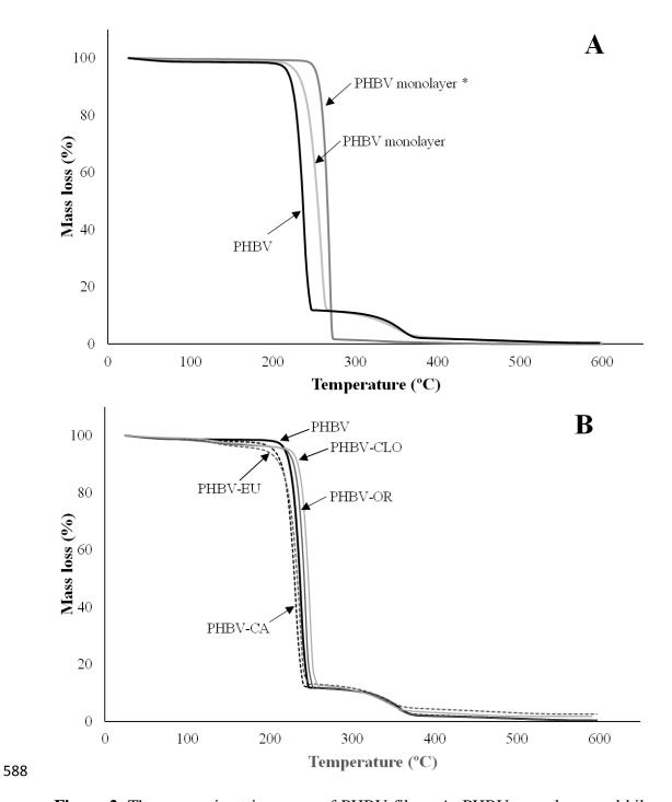
Figure 2. Thermogravimetric curves of PHBV films. A: PHBV monolayer and bilayer
