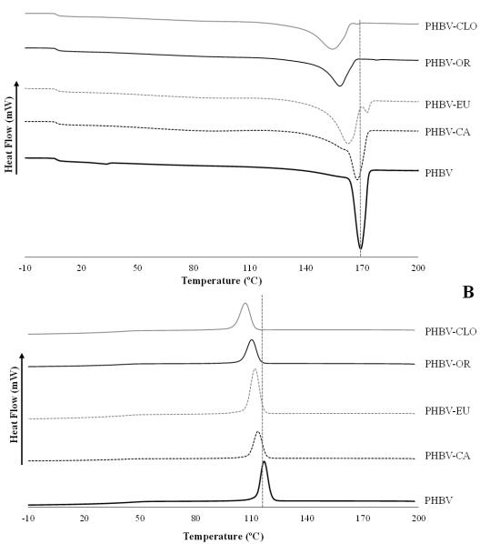
Figure 3. DSC thermograms for the first heating scan (A) and the cooling scan (B) of control PHBV film and with active compounds (CA: carvacrol, OR: oregano essential
