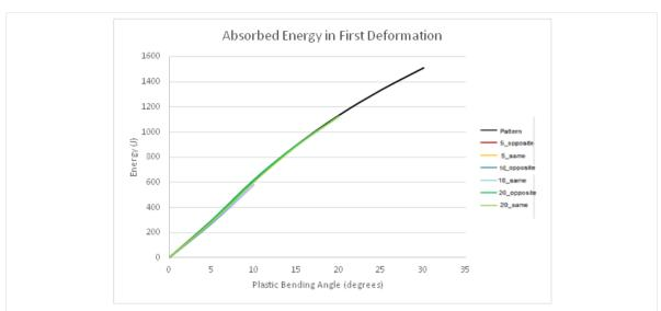
Fig. 1 – Absorbed plastic energy in STEP 1 deformation.
