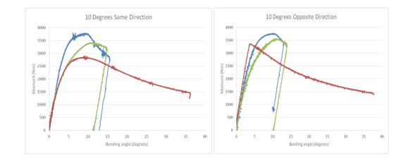
Fig. 3 – Moment – Bending angle. 10 degrees first deformation.
