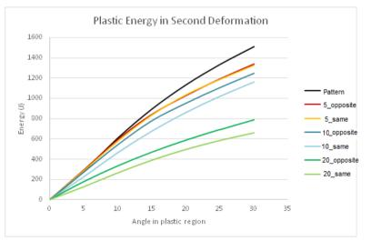
Fig. 5 – Absorbed plastic energy in second deformation.
