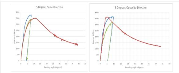
Fig. 2 – Moment – Bending angle. 5 degrees first deformation.
