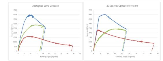
Fig. 4 – Moment – Bending angle. 20 degrees first deformation.
