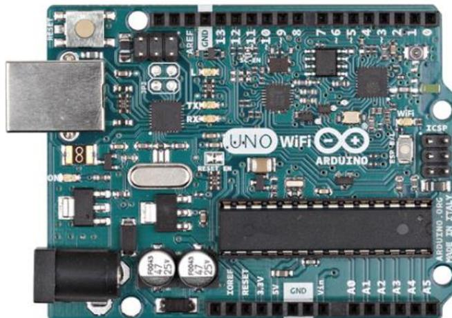
**Figura 4.2.1.8** Arduino Uno Wifi Shield.
