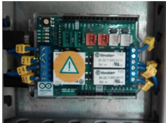
Figura 5.1.1 Arduino 4 Relays Shield
