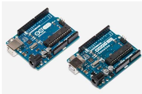
**Figura 2.2.2** Microcontrolador Arduino genuino UNO.
