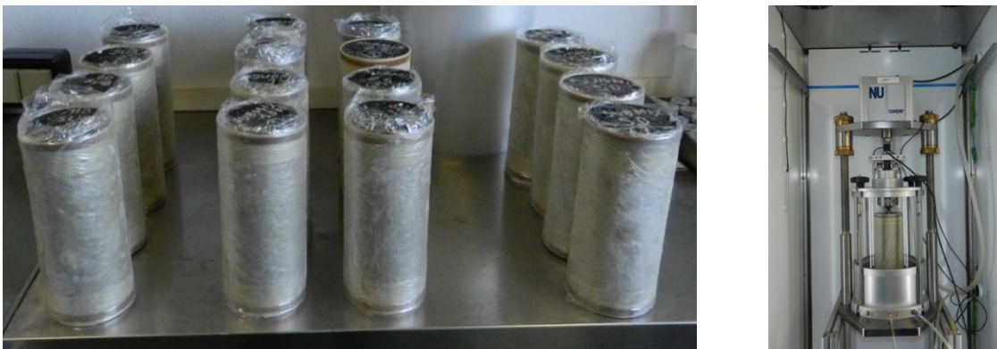
Figure 2. (a) Cylindrical Specimens Ø 100 mm H 200 mm (b) Cyclic Load Triaxial Test.
