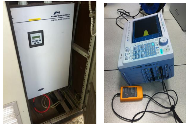
Fig. 4. Details of the field tests: soft-starter, current clamp and waveform recorder.
