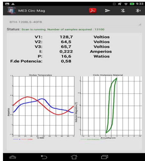
Fig. 10. Series-parallel II magnetic circuit test results.
