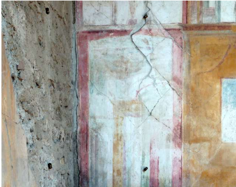
Figure 3: Dataloggers (small black pieces) mounted at Ariadnas house at Pompeii (Italy)
