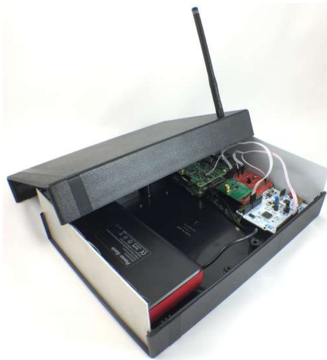
Figure 9: Low-power gateway prototype
