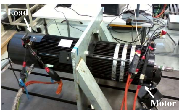
Fig. 3. Experimental test stand comprising two motors having the same characteristics coupled back-to-back.
