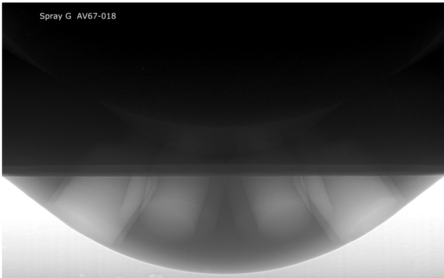
Figure 3.21: One of the 1800 images taken for tomographic reconstruction for one of the Spray G injectors (AV67-018).
