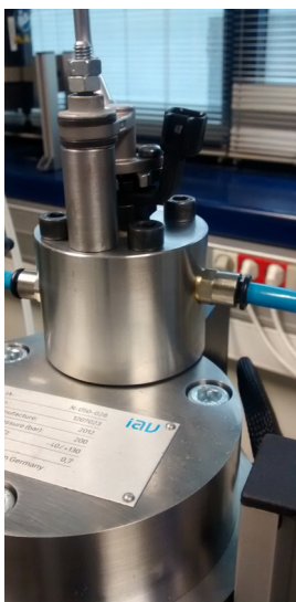
Figure 3.8: Injector, injector holder and IAV rate meter used in the experimental set-up.
