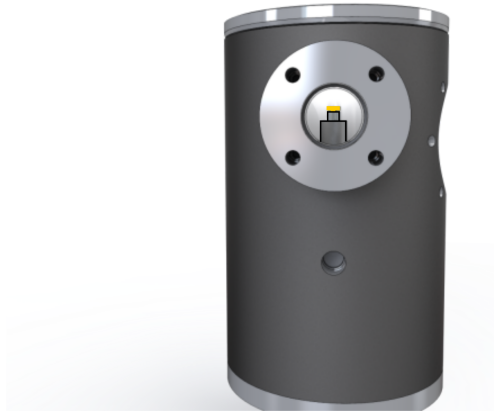
Figure 3.11: Render of the rate of momentum test rig showing the piezoelectric sensor through the optical access.
