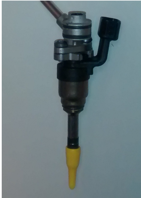
Figure 3.1: Picture of the Delphi Spray G injector AV67-026 with inlet fuel feed (cast rail) mounted.
