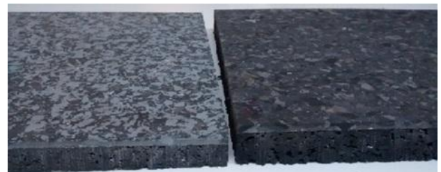
Fig. 5. Final products of thicknesses 18 and 22 mm.
