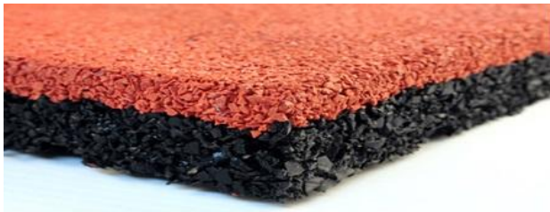
Fig. 4. Recycled rubber for technical flooring.
