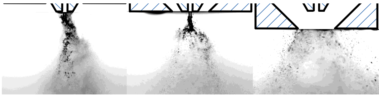
(c) Condition 3: Q_a / Q_w = 3800 (Nozzle cover position 1 to 3 from left to right)
