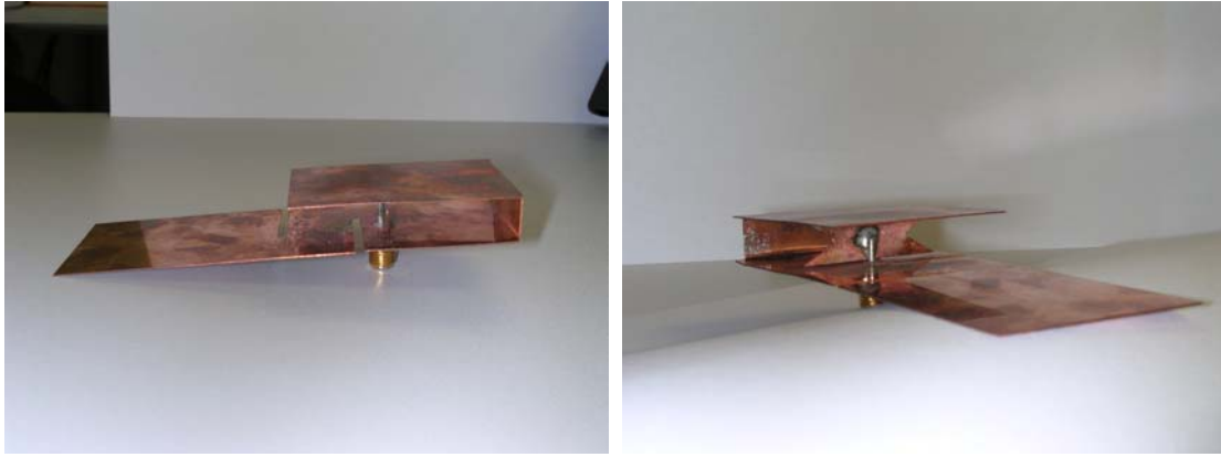
Figure 6.18 Photographs of the prototype of the slotted folded radiating ground plane fed with a bow-tie shaped monopole.
