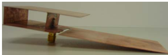
Figure 6.12 Prototype of the folded slotted radiating ground plane fed with a rectangular monopole.
