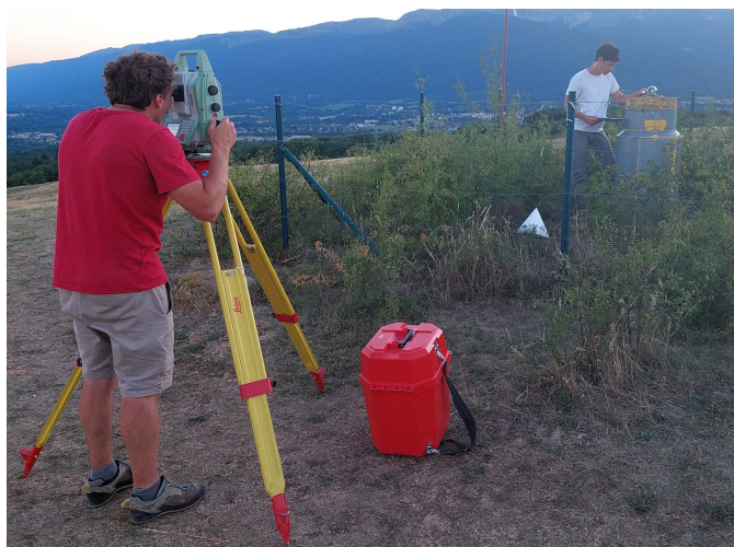
Fig. 9. Determining antenna height above pillar by Total Station.
