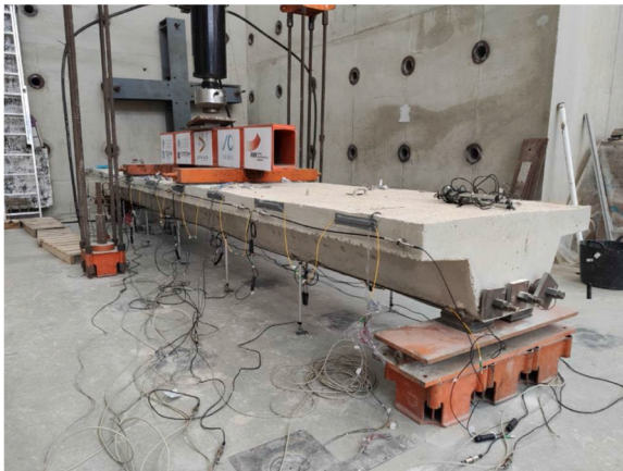
Fig. 9. Set up of the Four-point bending test.
