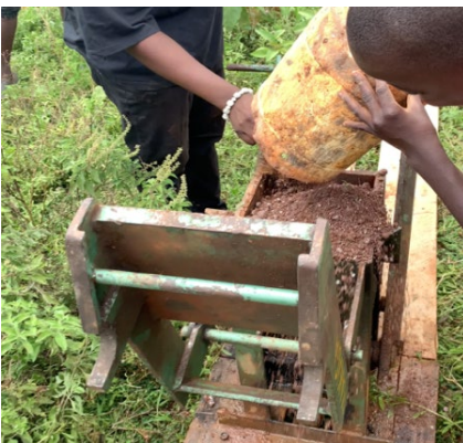
Fig. 9 – Infilling process of the “Makiga” CEB Press.
